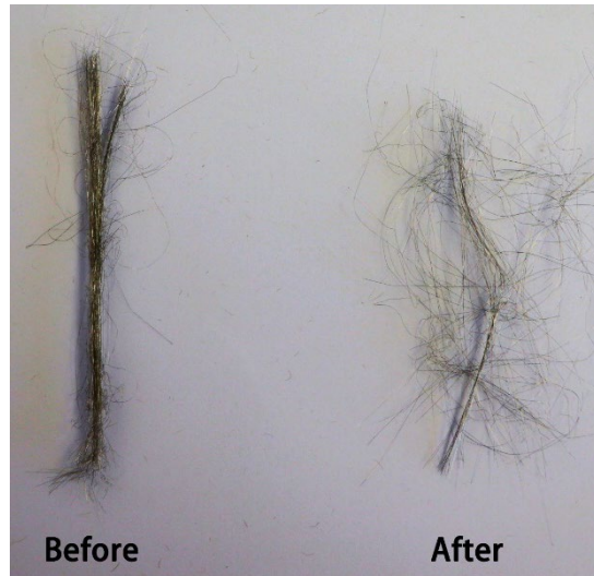
Left: Nickel strands as supplied | Right: Nickel strands ready to use
