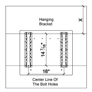
2. *Mount the Hanging Bracket:* Center the hanging bracket along the line marking you just made. Using the information in the table below, mount the bracket to the wall using the <sup>3</sup>/<sub>8</sub>"-diameter lag bolts following the bolt manufacturer's requirements (bolts are not provided). Recommended bolt length is minimum 3" but may need to be longer depending on project design needs.
