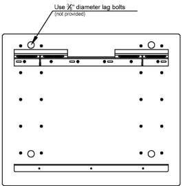
NOTE: To ensure the fireplace can be installed tightly to the wall, make sure the bolt doesn't stick out more than 5/8" from the wall.
