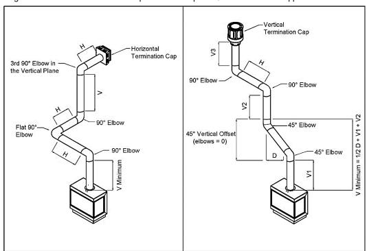
TERMINATION CAP NOTE: Low Profile Termination Cap and Sconce Termination Cap can negatively impact flame appearance and are not recommended for use with the fireplace.
