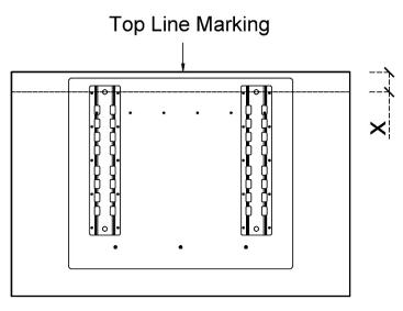
2. *Mount the Hanging Bracket*: Center the hanging bracket along the line marking made in Step 2.1. Using the information in the table below, mount the bracket to the wall using the <sup>3</sup>/<sub>8</sub>"-diameter expansion bolts following the bolt manufacturer's requirements (bolts are not provided). Recommended bolt length is minimum 3" but may need to be longer depending on project design needs.
