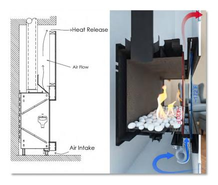
The fans need air from the room where the fireplace is located or from an alternate interior space. This requires an air intake, opening, below the fireplace to allow air to the fans.
