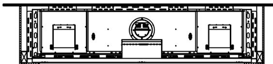
The valve can be moved 36" from the center of the fireplace in any direction
