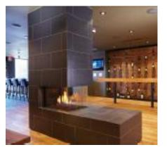
• **Floating Wall:** A floating wall can offer a creative alternative for incorporating the heat release and air intake (for double glass barrier) into one seamless design.
