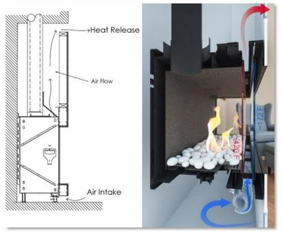
The heat travels up into the fireplace chase through openings on the top of the firebox, and then moves out into the room through the heat release. The fans need air from the room where the fireplace is located or from an alternate interior space. This requires an air intake, opening, below the fireplace to allow air to the fans.
