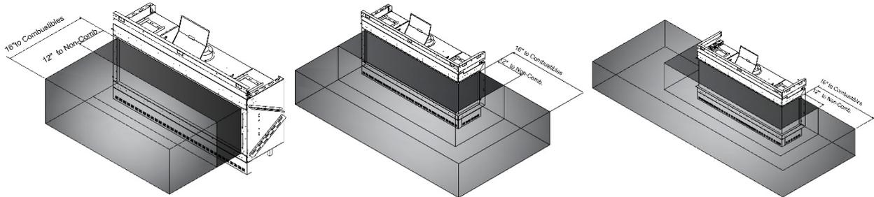
Materials (including combustible flooring and combustible finish material) are permitted below and around the viewing area clearance zone.
