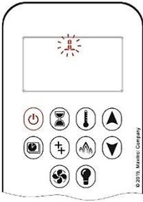
1. Press the
