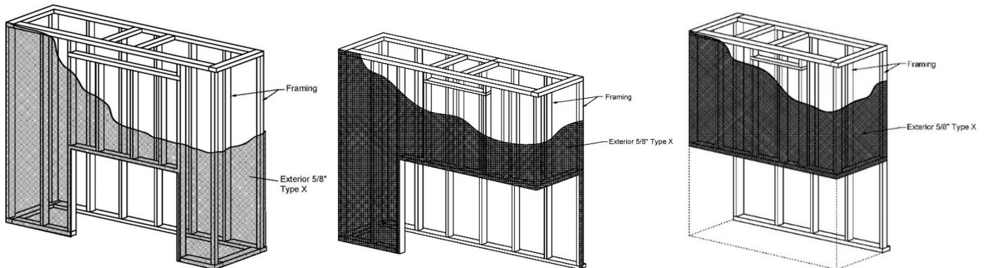
**!** NOTE:  $\frac{5}{8}$ " Type X Drywall (or equivalent) is not required on the exterior portion of an insulated outside-facing wall.
